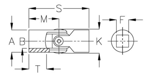
$\begin{array}{lll} A & = 63 \\ F & = 32 \\ K & = 65.0 \\ M & = 83 \\ MD \max N m = 250 \\ s & = 166 \\ T & = 50 \\ \end{array}$
